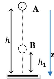
$$dW(\vec{f}) = m\vec{g}\vec{v}dt = mgvdt = mg\left(\frac{g}{k}(1 - \exp(-kt))\right)dt = \frac{mg^2}{k}((1 - \exp(-kt)))dt \quad (0,5)$$
