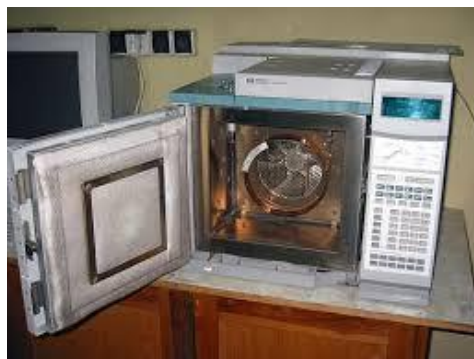
Four thermostaté contenant la colonne
