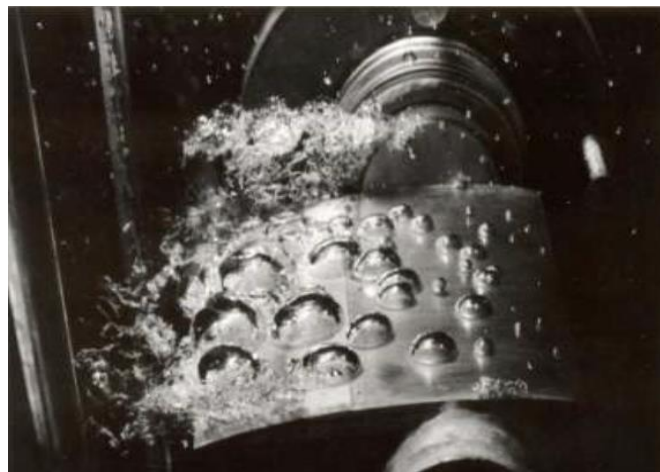
Figure 4. Bubble cavitation on a blade profile
