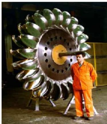
Figure c.3 Haute chute : turbine Pelton
