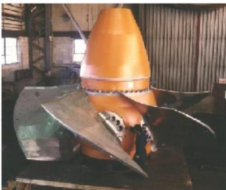
Figure c.1 Basse chute : turbine Kaplan
