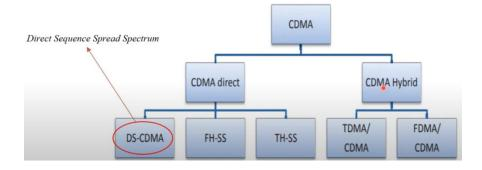
In this chapter we focus on the widely used Direct Sequence Spread Spectrum (DS-CDMA)
