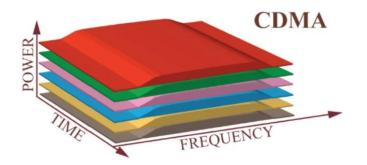
CDMA uses **the spread spectrum techniques**; the principle is to spread a signal over a wider frequency band using unique spreading code.
