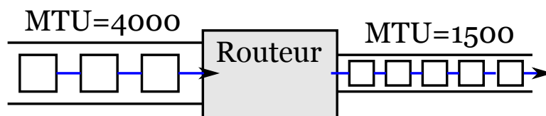
FIGURE 3.6: Fragmentation des datagrammes IP.
