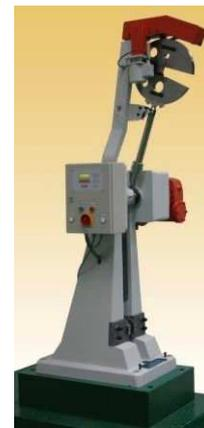
Figure 14. Machine mouton de Charpy
