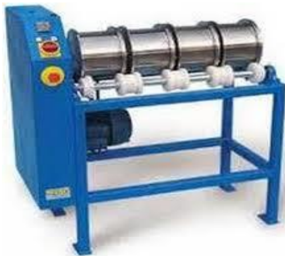
Figure IV.1: Appareil Micro Deval
