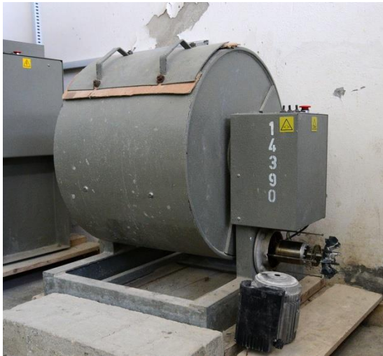
Figure IV.3: Appareil Los Angeles
