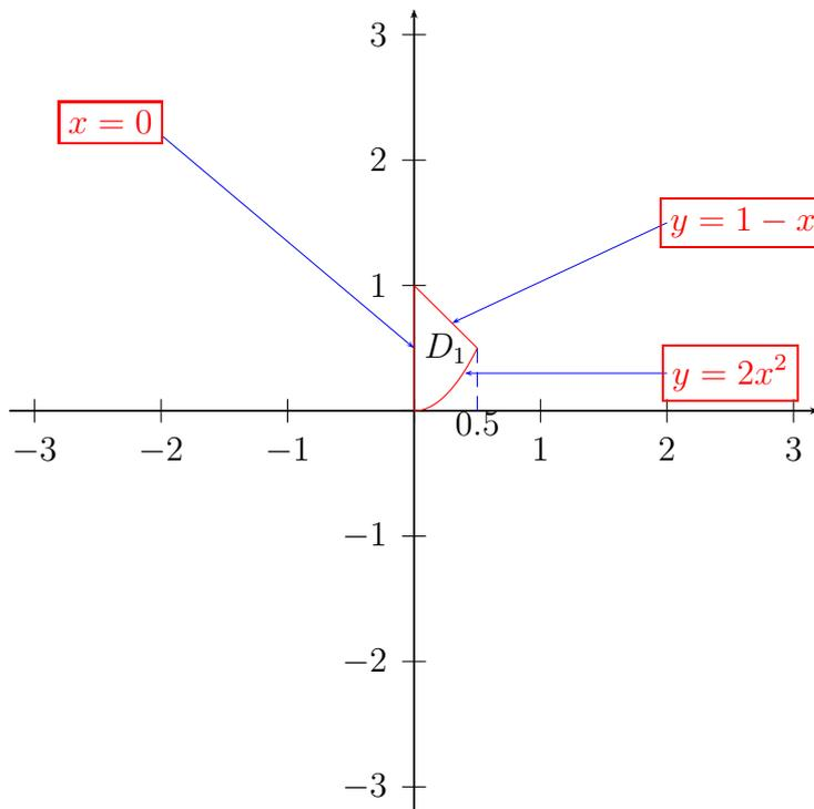
$$\int \int_{D_2} y\sqrt{x} dx dy = \int_0^1 \left[ \int_0^{1-x} yx^{\frac{1}{2}} dy \right] dx$$
