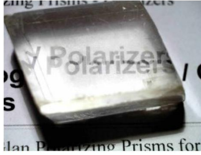
Figure III.1: Observation of the doubling of the image of an object viewed through a calcite crystal showing birefringence.
