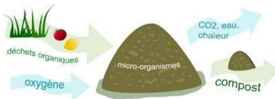
Figure III.5. Principe du compostage
