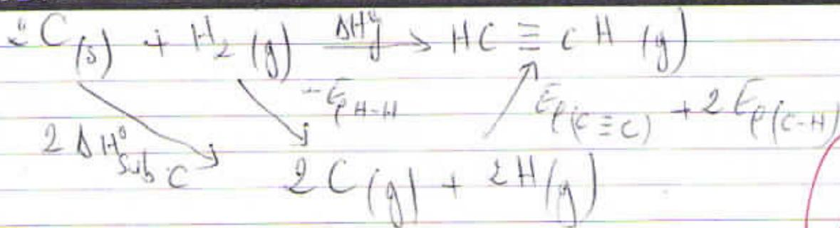
$$\Delta H_f^\circ C_2H_2 = 2\Delta H_{sub}^\circ C - E_{H-H} + E_{C \equiv C} + 2E_{C-H}$$
