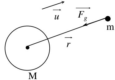
$$\begin{aligned} \overrightarrow{F}_g &= -\overrightarrow{\text{grad}} E_p(r) = -\frac{dE_p}{dr} \overrightarrow{u} \\ \Rightarrow \quad \frac{dE_p}{dr} &= G \frac{M \, m}{r^2} \\ E_p(r) &= \int G \frac{M \, m}{r^2} dr \\ \Rightarrow \quad E_p(r) &= G \frac{M \, m}{r} + \text{cste} \end{aligned}$$
