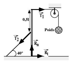
$T_1$  = 100 N ,  $T_2$  = 261 N ,  $R_t$  = 100 N  $\,$  et  $\,R_n$  = 368 N  $\,$
