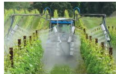
Two-row electrostatic spray booms create a targeted 50-micron fog.
