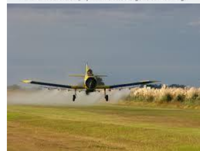
Two-row electrostatic spray booms create a targeted 50-micron fog.
