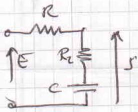
$$F(j\omega) = \frac{S}{E} = \frac{R_2 + \frac{1}{j\omega C}}{R_1 + R_2 + \frac{1}{j\omega C}} = \frac{1 + jR_2\omega C}{1 + j(R_1 + R_2)\omega C}$$
