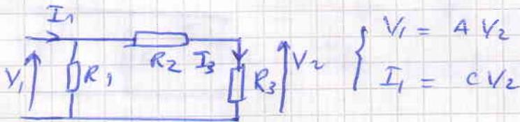
$$V_1 = A V_2$$
