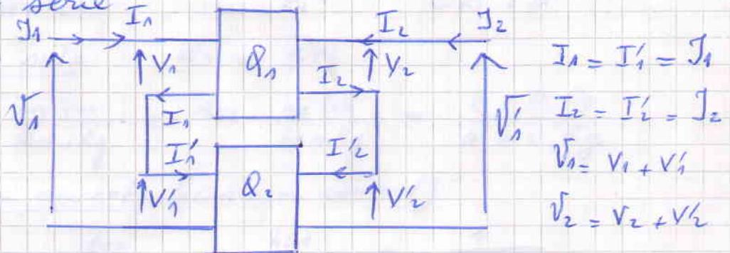
$$\begin{aligned} I_1 &= I_1' = I_1 \\ I_2 &= I_2' = I_2 \\ V_1 &= V_1 + V_1' \\ V_2 &= V_2 + V_2' \end{aligned}$$
