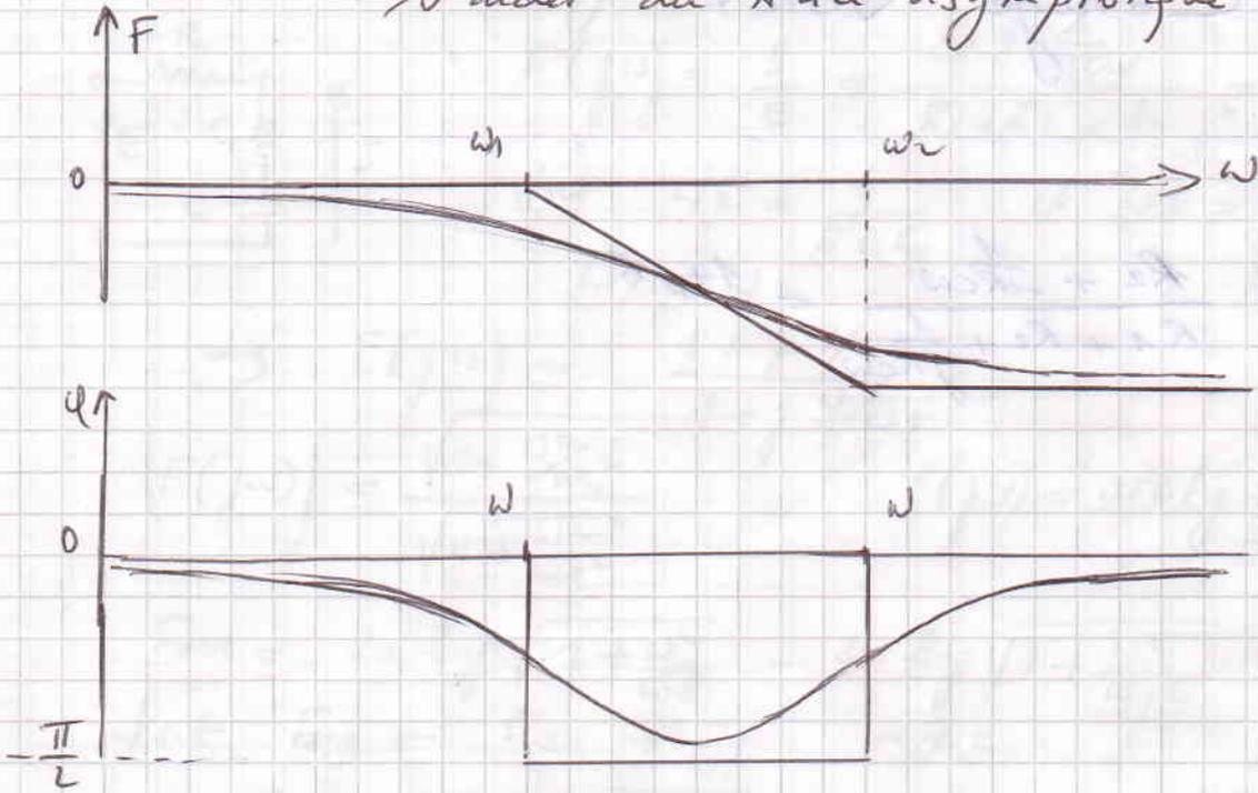
$$\omega = \omega_1, \quad F = 20 \log \sqrt{1 + \left(\frac{R_2}{R_1 + R_2}\right)^2} - 20 \log \sqrt{1 + 1}$$
