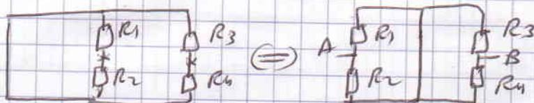
$$R_{th} = (R_1 \parallel R_2) + (R_3 \parallel R_4)$$
