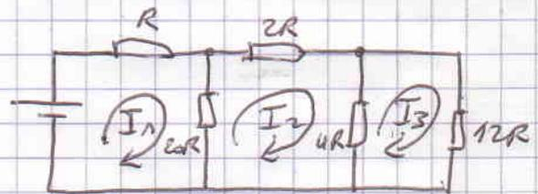
Ex  $\left\{ \begin{array}{l} E = 20R(I_1 - I_2) + RI_1 \\ E = RI_1 + 2RI_2 + 4R(I_2 - I_3) \\ 0 = 20R(I_1 - I_2) - 2RI_2 - 12RI_3 \end{array} \right.$
