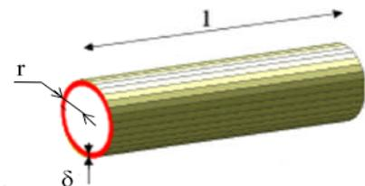
$$S_\delta = \pi[r^2 - (r-\delta)^2] = \pi\delta(2r-\delta) \quad \text{et} \quad R_\delta = \frac{l}{\sigma S_\delta}$$
