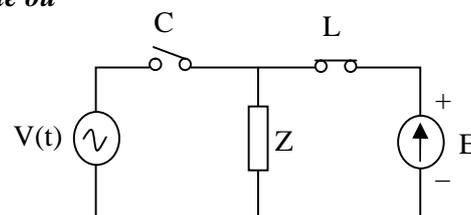
$$V_L = L \frac{dI_L}{dt} = jL\omega I_L \Rightarrow V_L = 0 \quad : \text{Circuit fermé}$$
