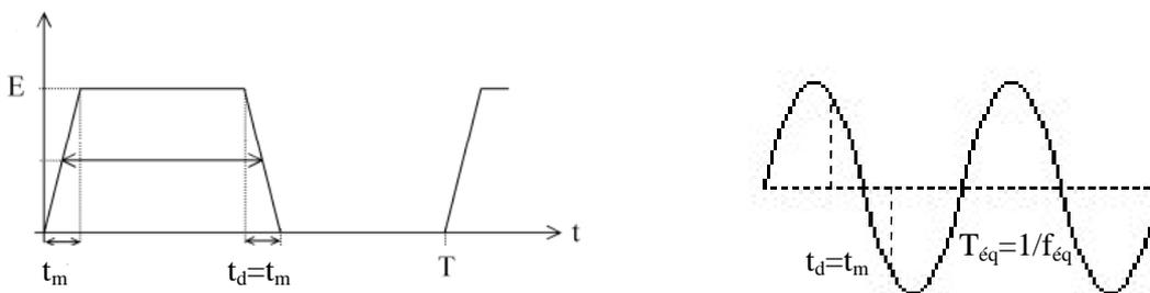
$$T_{eq} = 3t_m \Rightarrow f_{eq} = \frac{1}{T_{eq}} = \frac{1}{3t_m}$$
