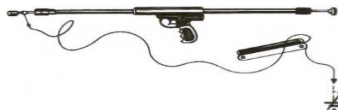
Figure VII.16 : Fusil lance câble
