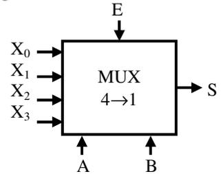
$$S = \overline{E}\overline{B}\overline{A}X_0 + \overline{E}B\overline{A}X_1 + \overline{E}\overline{B}AX_2 + \overline{E}BAX_3$$
