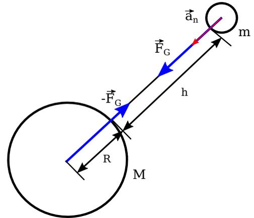
FIGURE 3.6 – Forces de gravitation
