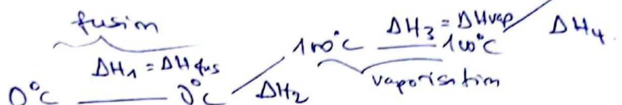
$$\Delta H_T = \Delta H_1 + \Delta H_2 + \Delta H_3 + \Delta H_4$$
